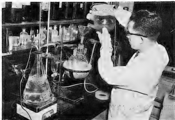
FIG. 4 - A MIXTURE OF FISH-OIL GLYCERIDES BEING HYDROLYZED BY SODIUM-REDUCTION REACTION TO PREPARE FATTY ALCOHOLS.
